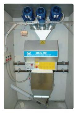
The operation unit of the weigher has a display in which the total amount of weighed feed can be read in grams, kilos or tons. The operation unit is mounted in a dustproof case. The required portion of
